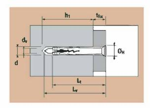
d<sub>0</sub> = plug diameter = hole diameter
